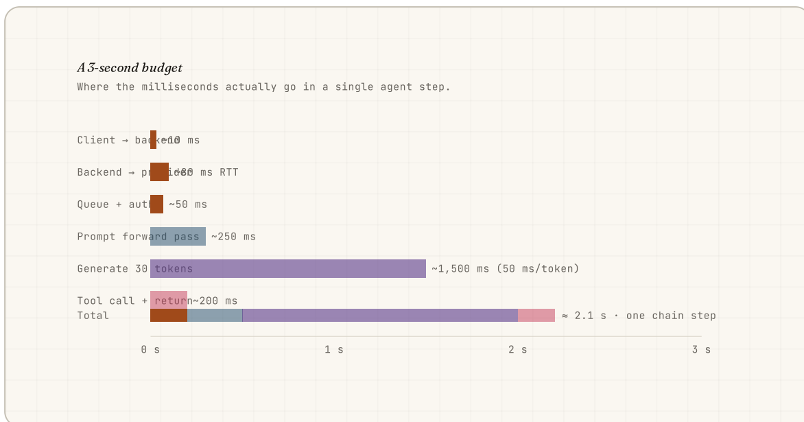
FIGURE 33.1 A three-second response budget, broken into pieces. Network round-trips, queue wait, prompt-processing pass, and per-token generation each take a real share. Add a tool call and the budget collapses.
